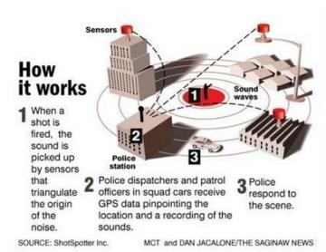
**Gunshot detector:** Cities and law enforcement can use gunshot detectors to identify where in the city shots are fired. They do this by placing sensors with microphones around the city, then when a shot is detected from more than one sensor, law enforcement can be notified. The more sensors that pick up the sound, the better they can pinpoint the exact location of the gunshots. The goal of these gunshot detectors is to quickly respond to violent crimes.
